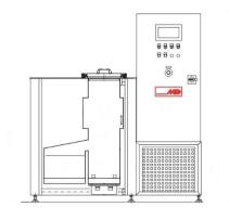
Mono-solvent (M) machines incorporate a liquor-vapour stacked, process with closed vapour generator. The cleaning process involves ultrasonic, liquid cleaning immersion followed by vapour rinsing.
