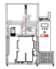
Co-solvent (C) machines use a traditional, twinsump, process layout and two-axis handling system, providing boiling liquid pre-wash followed by ultrasonic liquid immersion clean and vapour rinse.
