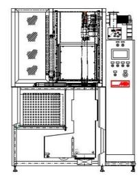
Mono-solvent (M) machines incorporate a stacked, liquor-vapour process with closed vapour generator and single-axis, basket handling system. The cleaning process involves ultrasonic, liquid cleaning immersion followed vapour by rinsing.
